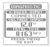
used to evaluate the health of the battery by showing the present voltage. Voltage can also be viewed in the Trip Log view.
